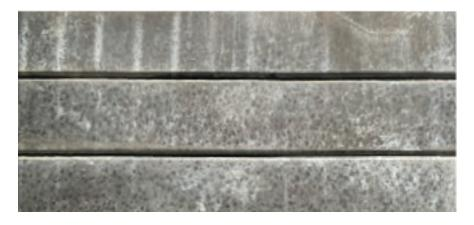
All concrete products are susceptible to Lime Bloom which can appear on your concrete sleepers as thin white patches. Lime Bloom is temporary and typically disappears as a result of normal weathering.
